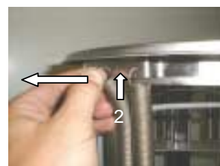
Figure 5-6-3-4: Unhooking the springs at the top
