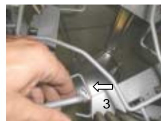
Figure 5-6-2-3: Bore holes (3) in the base plate
