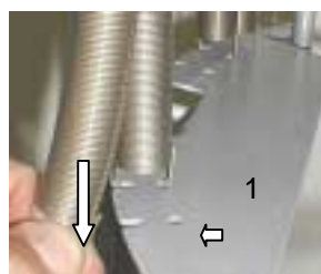
Figure 5-6-3-3: Unhooking the springs at the bottom
