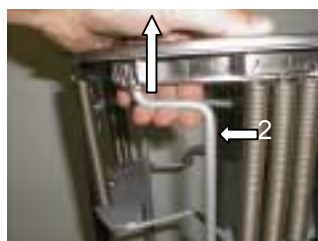
Figure 5-6-2-2: Lift the adjustment rod (2)
